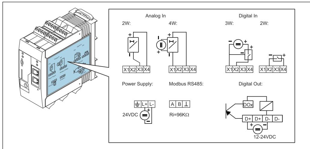
9 Labeling on the housing for terminal assignment
