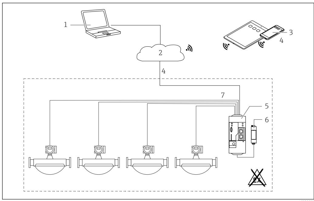
4 System architecture of a Fieldgate FXA42 with a pulse counter
