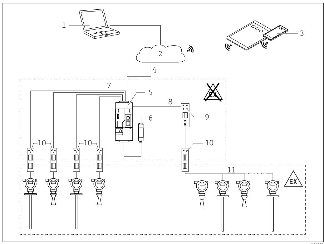
7 System architecture of a Fieldgate FXA42 with HART Multidrop
