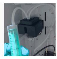
■ 12 Draining the SPx sample hose and photometer
