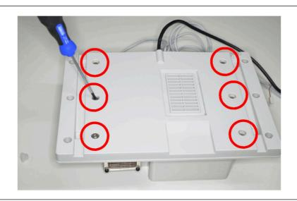
**■** 14 Removing the cooling module cover
