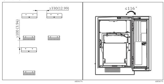
■ 10 Minimum spacing required for installation. Unit ■ 11 Maximum opening angle of measurement mm (in)
