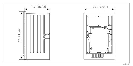
$\blacksquare$  14 Open installation. Unit of measurement mm (in)
