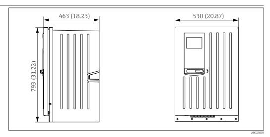
■ 13 Enclosed installation. Unit of measurement mm (in)
