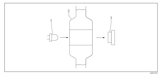
■ 1 Colorimetric measuring principle
