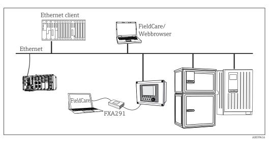
■ 21 Modbus TCP or EtherNet/IP or PROFINET
