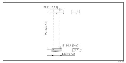
Dimensions of holder. Unit of measurement mm (in)
