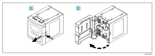
🖻 19 Access to terminal compartment: single DIN rail housing unit
