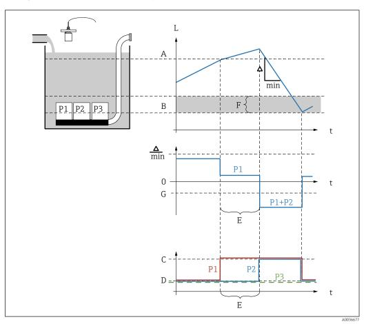
Configuration of the pump control system (function: Pump rate control)
