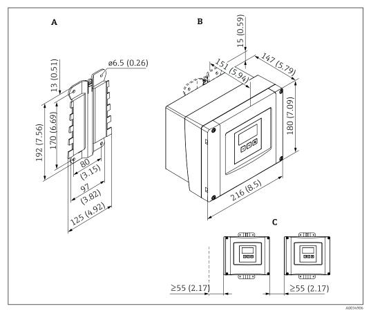
■ 6 Dimensions of Prosonic S with polycarbonate field housing. Unit of measurement mm (in)
