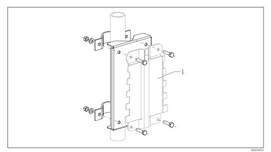
**1** 8 Mounting plate for mounting the polycarbonate field housing on a post
