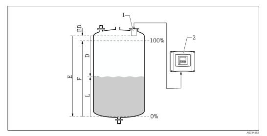
■ 47 Empty and full calibration for level measurement
