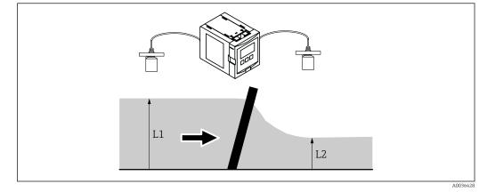
Operating principle of the rake control function
