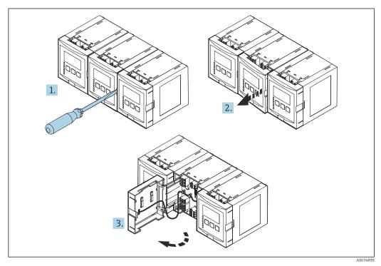
■ 20 Access to terminal compartment: several DIN rail housing units mounted side by side
