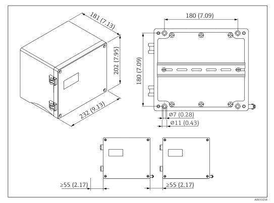
Dimensions of Prosonic S with aluminum field housing. Unit of measurement mm (in)
