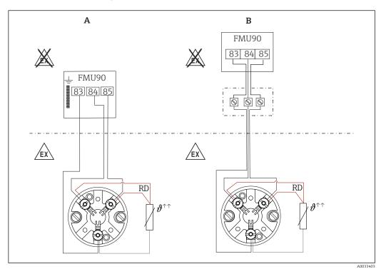
Connection of the Omnigrad S TR61 temperature sensor in hazardous areas
