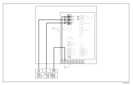
■ 22 Connection of the power supply in the polycarbonate field housing
