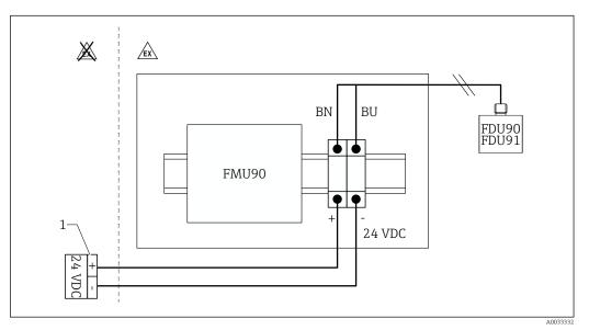
31 Connection of the sensor heater in the aluminum field housing
