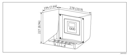
☑ 72 Weather protection cover for polycarbonate field housing. Unit of measurement mm (in)
