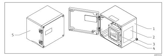
Access to terminal compartment in aluminum field housing
