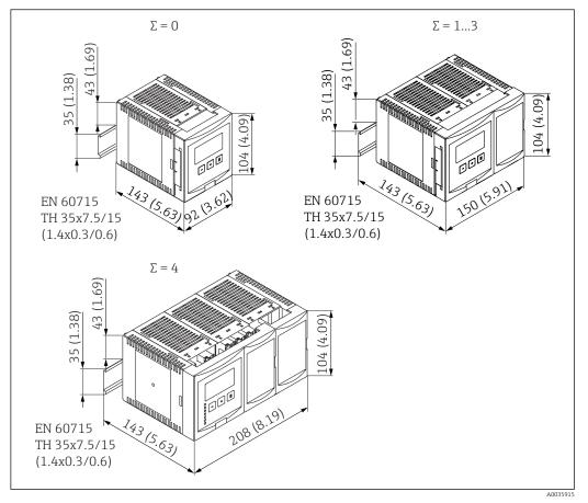
E 11 Dimensions of Prosonic S with DIN rail housing;  $\Sigma$ : number of additional connection modules. Unit of measurement mm (in)
