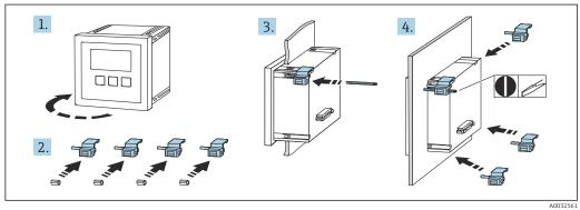
■ 15 Installing the remote display and operating module
