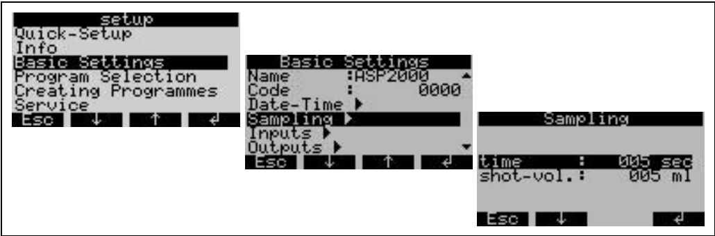
Fig. 14: ASP Inline sampling menu structure (via ASP Station 2000 control unit)
