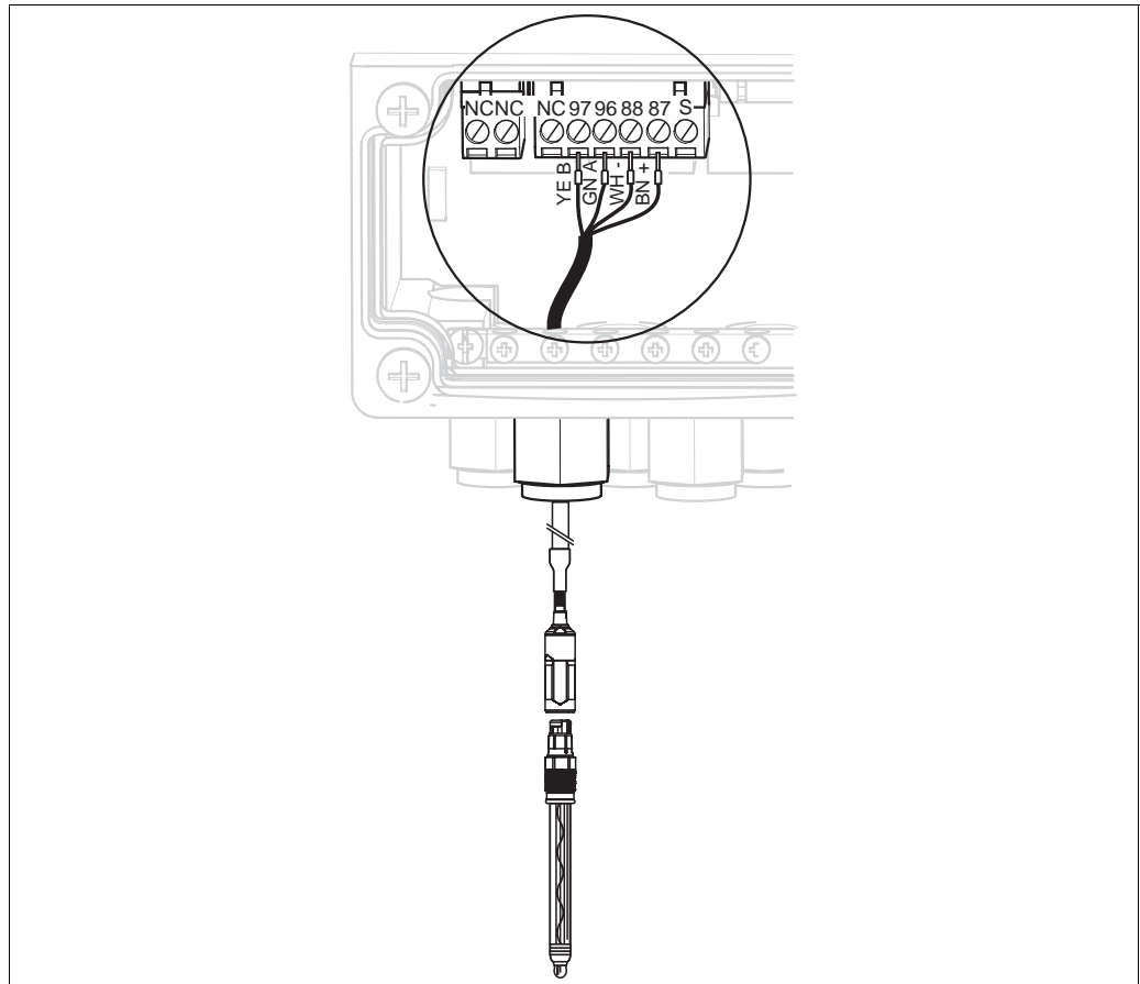
Fig. 31: Connecting digital sensors with Memosens technology
