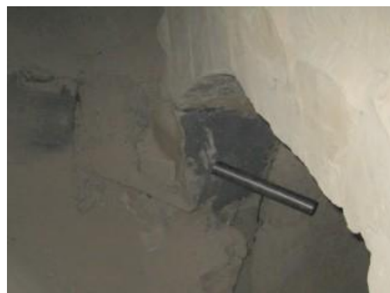
Fig. 24: Protection tube covered with refractory concrete inside the kiln (example)
