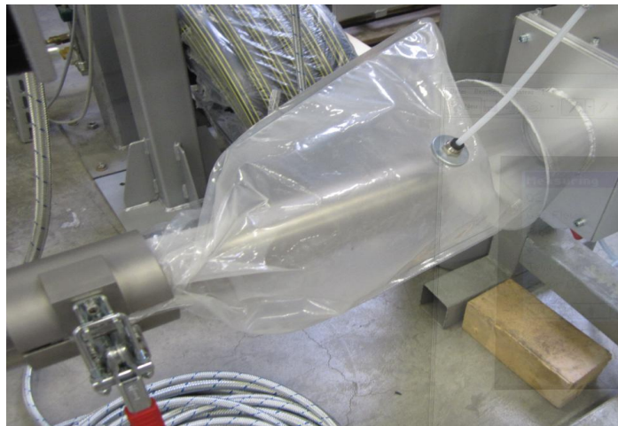
Fig. 53: Sealing clamp with test gas inlet bag.
