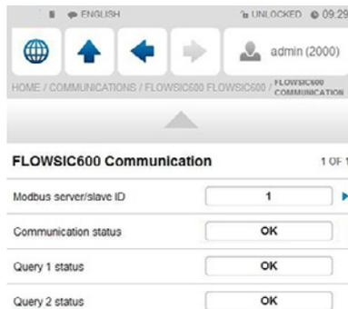
Fig. 29 - Voce di menu "Communication -> Flowsic600-XT Flow Meter -> FLOWSIC600-XT Communication"
