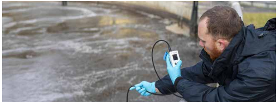
Oxygen measurements in an aeration basin
