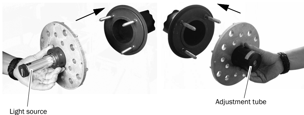
Fig. 7: Aligning the flange using an optical adjustment device
