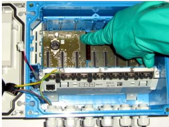
Figure 7: Installation of extension backplane module
