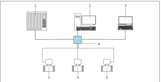
Options for remote operation via Modbus TCP over Ethernet - 100 Mbit/s: Star topology
