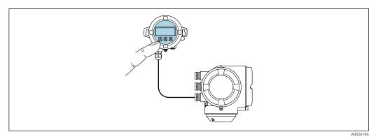
Operation via remote display and operating module DKX001
