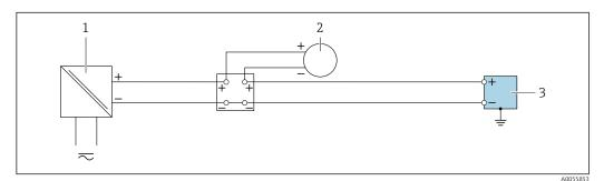
■ 13 Connection example for 4 to 20 mA current input
