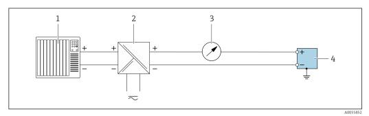
■ 12 Connection example for 4 to 20 mA current output (passive)
