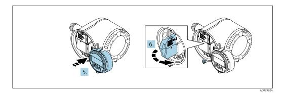
5. Attach the holder to the edge of the electronics compartment.
