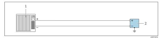
Connection example for pulse output/frequency output/switch output (active)
