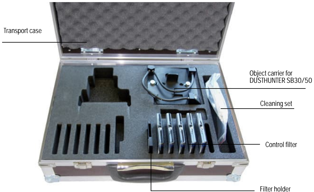
Fig. 18: Components of the equipment for the linearity test
