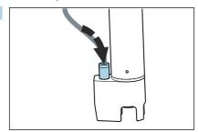
Connect the hose for the compressed air supply (to be provided onsite) or compressor to the hose connection of the cleaning unit.
