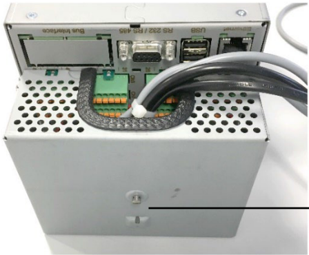
Terminal cover on Memograph M RSG45 zinc diecast version
