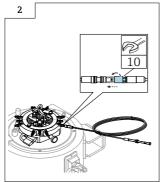
► Tighten the locking sleeve of the cable extension to the stop.
