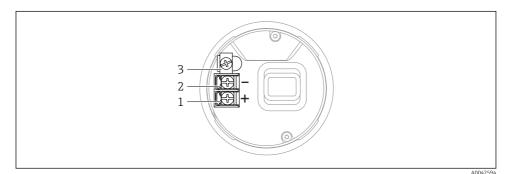
$\blacksquare 1$  Connection terminals and ground terminal in the connection compartment
