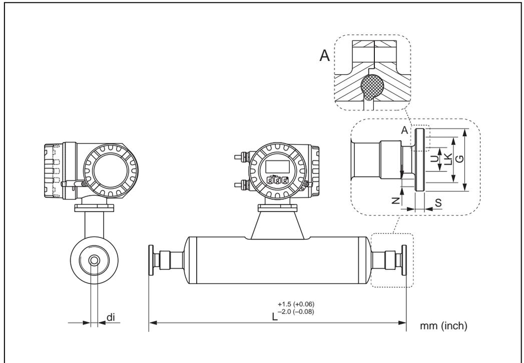
Detail A: The flange has the smaller groove for the O-ring on the sensor side. When mounting the sensor the corresponding flange must have accordingly a larger groove.
