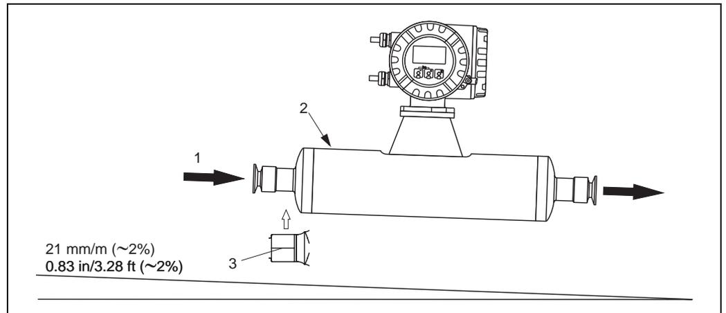
When lines are pitched in a specific direction and at a specific slope: as per hygienic guidelines (21 mm/m (0.83 in/3.28 ft) or approximately 2%). Gravity can be used to achieve complete drainability.
