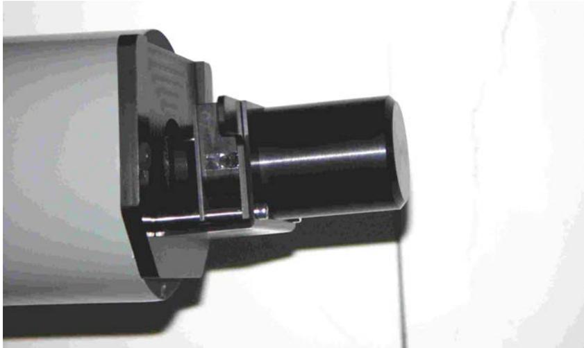
Fig. 42: Attach the test tool on the front of the sender/receiver unit.
