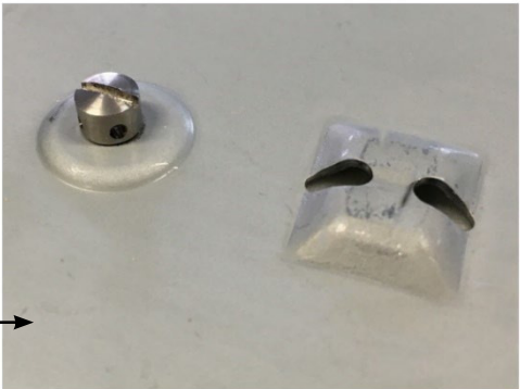
Fixing screw with hole for regulatory seals
