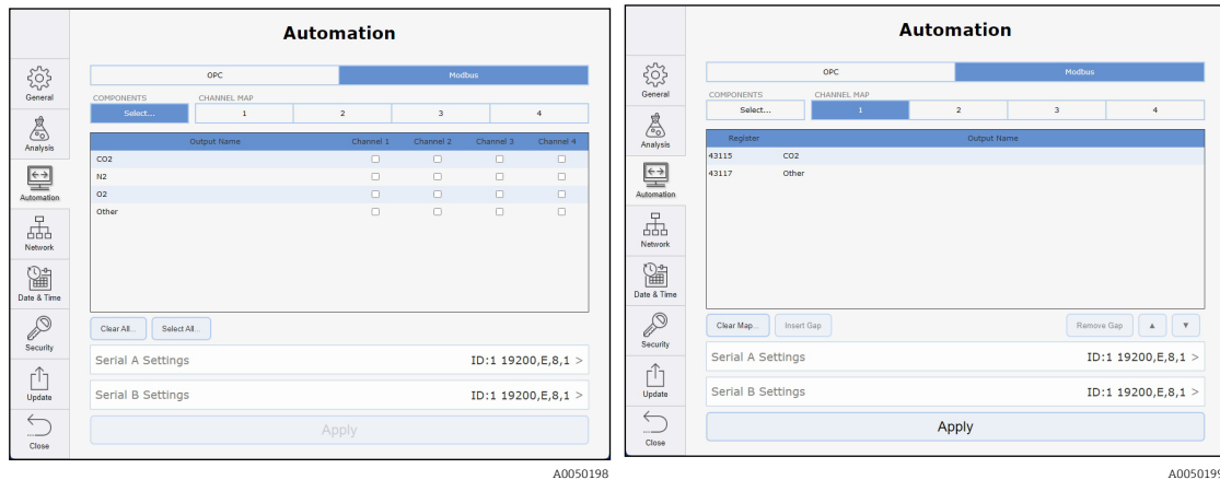
Figure 3. System settings – automation tab – Modbus (left), System settings – automation tab – Modbus channel map (right)
