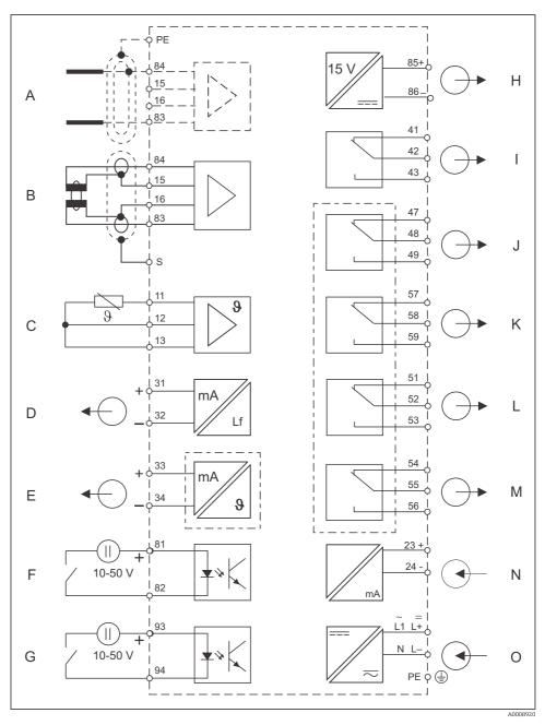
■ 7 Electrical connection of the transmitter
