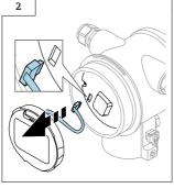
► Press the release mechanism and remove the display module.
