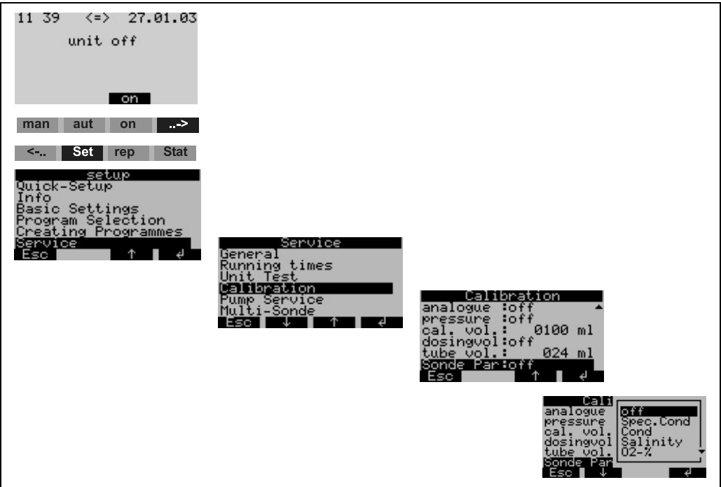
Fig. 20: Multi-parameter probe calibration
