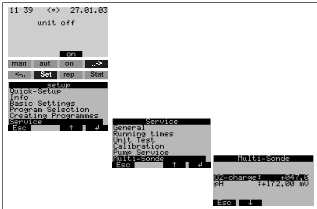
Fig. 21: Checking pH measurement (Sensor Check System)
