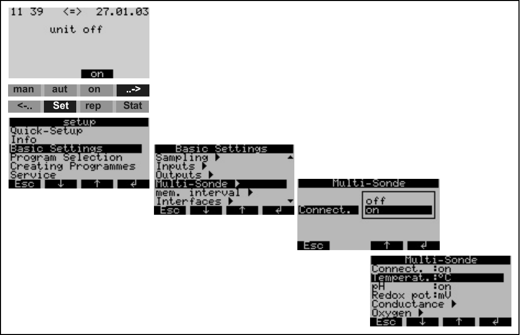
Fig. 23: Commissioning the multi-parameter probe (optional)
