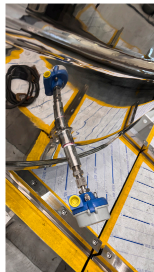
iTHERM ModuLine TM131 applied to PD Mixer
