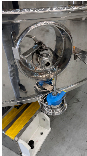
iTHERM ModuLine TM131 applied to PD Mixer
