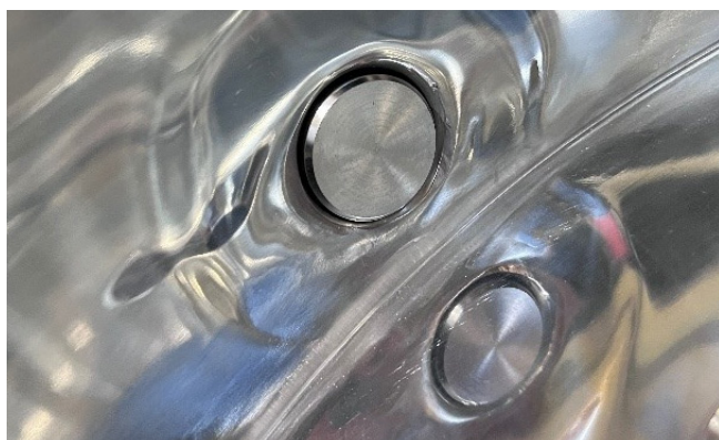
Sensor mounted in the wall of the mixer with an extremely short immersion length
