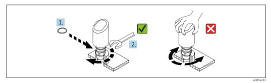
■ 2 Screwing in the device
