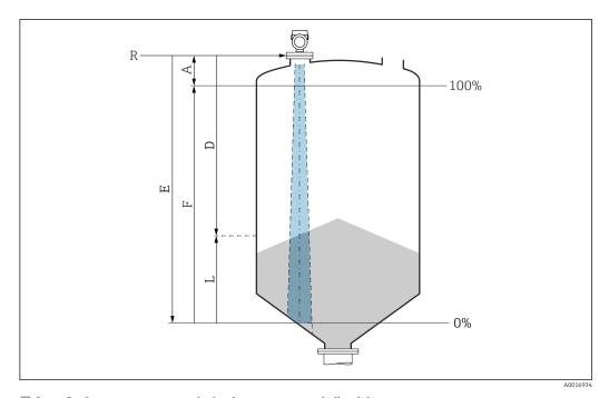
$\blacksquare$  9 Configuration parameters for level measurement in bulk solids
