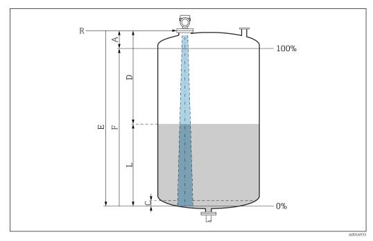
■ 8 Configuration parameters for level measurement in liquids
