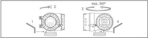
Fig. 1: Turning the transmitter housing
