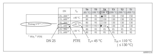
Fig. 3: Procedure for calculating the max. surface temperature
