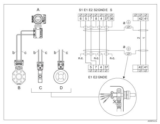
Fig. 6: Connection of remote version connecting cable
