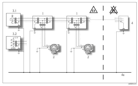
Fig. 5: Example for connecting potential equalization lines
