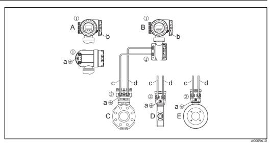
Fig. 4: Design of the measuring system, compact/remote version
