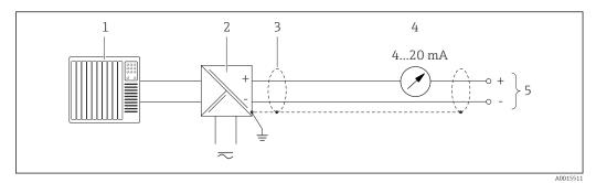
■ 1 Connection example for 4-20 mA HART current output (passive)
