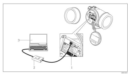
1 Service interface (CDI = Endress+Hauser Common Data Interface) of the measuring device
