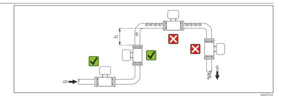
Preferably install the sensor in an ascending pipe, and ensure a sufficient distance to the next pipe elbow:  $h \ge 2 \times DN$
