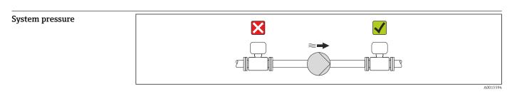
Never install the sensor on the pump suction side in order to avoid the risk of low pressure, and thus damage to the liner.
