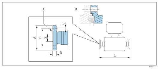
20 Detail X: Asymmetrical process connection; the part shown in gray is provided by the supplier.
