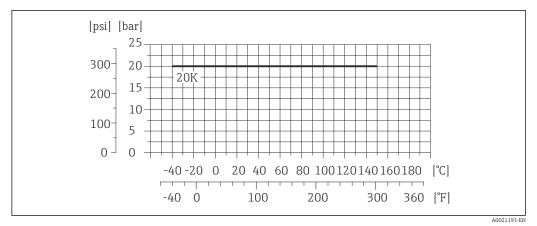
■ 15 Process connection material: stainless steel, 1.4404 (F316L)
