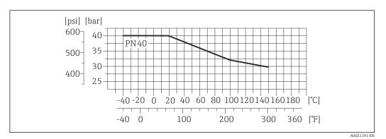
🛃 9 Process connection material: stainless steel, 1.4404 (F316L)
