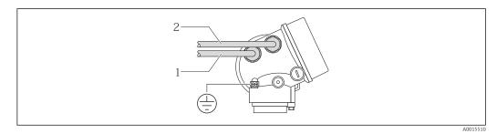
Cable entry for output 1 Cable entry for output 2 1 2
