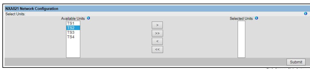
Assignation Tankvision Data Concentrator - Tank Scanner
