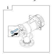
The fixing screw ( 26 mm (1.02 in)) (M3) is supplied in the kit.
