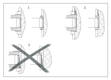
The adapter should be mounted in such a way, that it is flush with the inner vessel wall (1). Alternatively, the adapter can protude slightly into the process (2), as long as he stands no risk of being damaged by falling media. A recessed position (3) must be avoided, because media can accumulate there, impairing the function of the devices.
