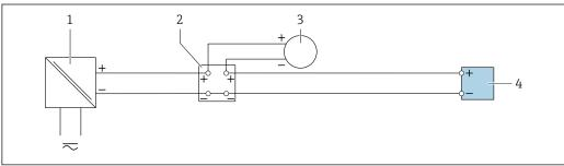
Connection example for 4 to 20 mA current input
