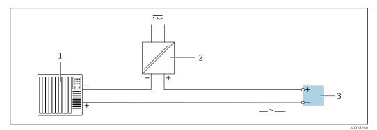
**₽** 21 Connection example for relay output (passive)
