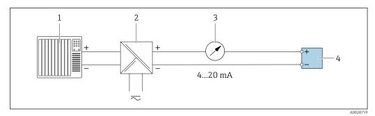
■ 18 Connection example for 4-20 mA current output (passive)
