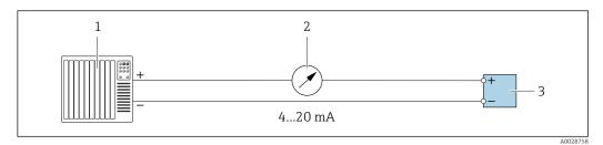
17 Connection example for 4-20 mA current output (active)
