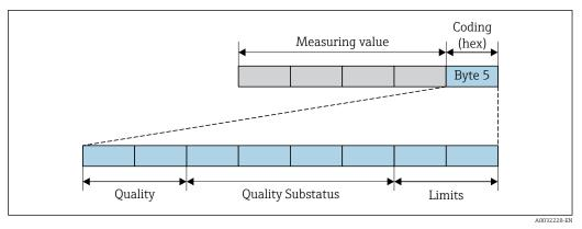
**■** 36 Structure of the coding byte
