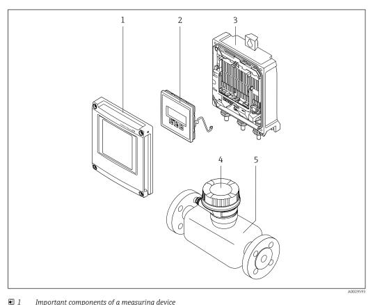
Important components of a measuring device
