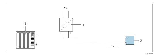
20 Connection example for switch output (passive)
