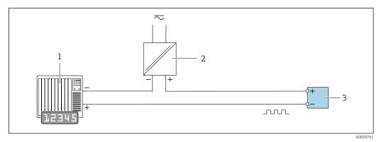
■ 19 Connection example for pulse/frequency output (passive)
