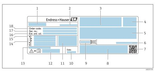
■ 3 Example of a transmitter nameplate
