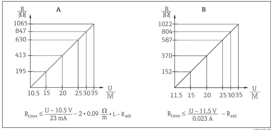
A FMX21 4 to 20 mA HART load chart for estimating the load resistance. Additional resistances, such as the resistance of the extension cable, have to be subtracted from the value calculated as shown in the equation.
