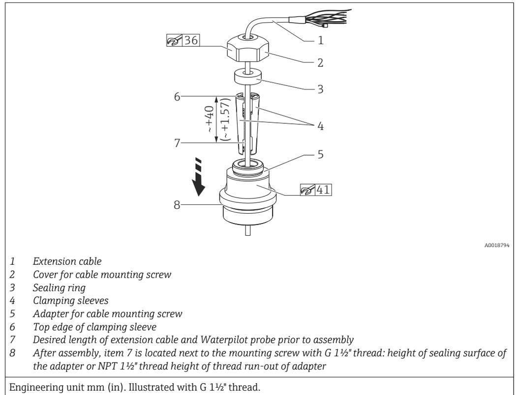
**i** If you want to lower the level probe to a certain depth, position the top edge of the clamping sleeve 40 mm (4.57 in) higher than the required depth. Then push the extension cable and the clamping sleeve into the adapter as described in Step 6 in the following section.
