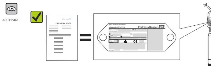
Do the data on the nameplate correspond to the order specifications and the delivery note?
