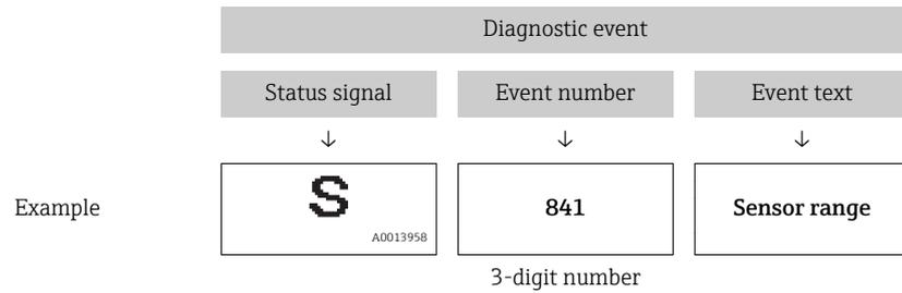
If two or more diagnostic events are pending simultaneously, only the diagnostic message with the highest priority is shown.
