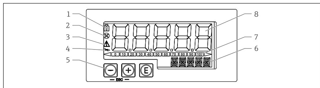
6 Display and operating elements of the process display unit
