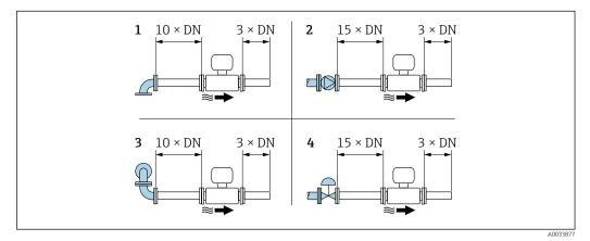
■ 6 Minimum inlet and outlet runs with various flow obstructions
