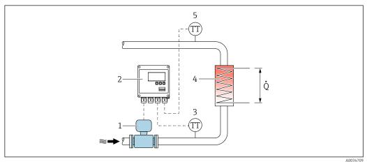
I Heat and cooling meter measuring system
