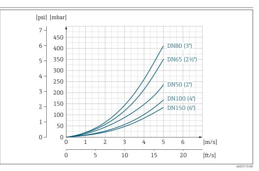
I4 Pressure loss DN 50 to 150 (2 to 6")
