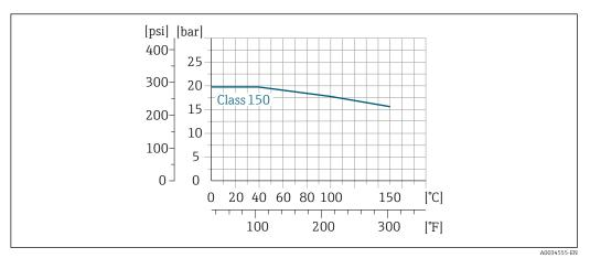
■ 11 With flange material A105; minimum process temperature  $\rightarrow$   $\square$  16
