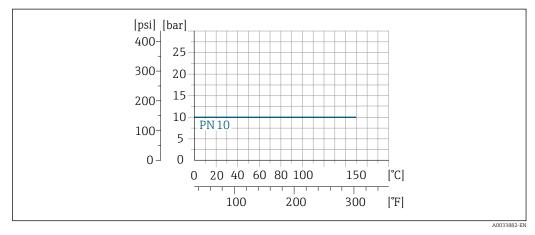
■ 13 With flange material 1.0038 (S235JR) and 1.4301 (F304); minimum process temperature  $\rightarrow$   $\triangleq$  16
