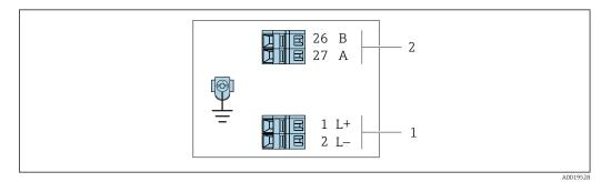
■ 3 Pulse/frequency output terminal assignment
