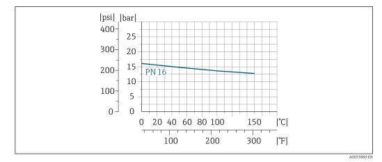
Lap joint flange DIN EN 1092-1Type 02Shape A, PN 16
