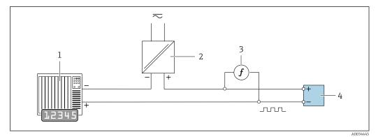
External verification of passive pulse/frequency output
