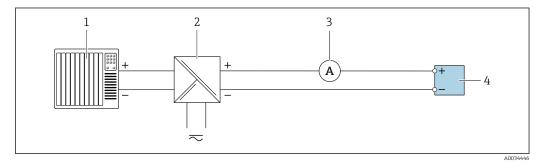
External verification of passive current output
