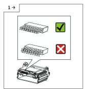
Check the male pin header strip of the electronics module before installation. The pins must not be bent.
