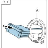
► When installing, slide the electronics module along the mounting guide rail (A) in the transmitter housing.
