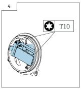
► Tighten the screws of the electronics module.
