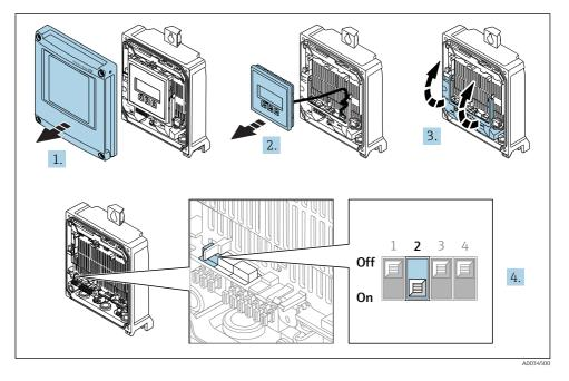
▶ Set DIP switch No. 2 on the I/O electronics module from **OFF**  $\rightarrow$  **ON**.
