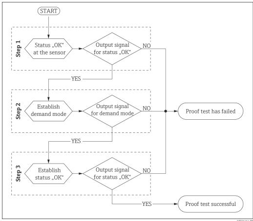
A demand mode or a fault takes absolute precedence over the proof test and in the measuring system safety path. For this reason, the demand mode must first be ended or the fault rectified before the proof test can commence. It is advisable to also check that the alarm relay (terminal 15 and 16) has not de-energized (no fault is present) at the start of the proof test (step 1).
