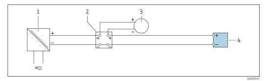
■ 15 Connection example for 4 to 20 mA current input
