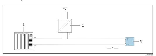
■ 13 Connection example for switch output (passive)
