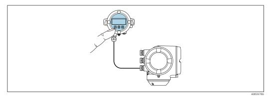
$\blacksquare$  35 Operation via remote display and operating module DKX001
