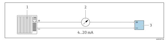
■ 10 Connection example for 4-20 mA current output (active)
