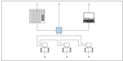
Options for remote operation via PROFINET network: ring topology
