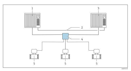
■ 25 Example of the layout of a redundant system (S2): star topology
