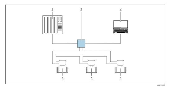
22 Options for remote operation via PROFINET network: ring topology
