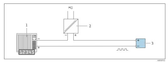
12 Connection example for pulse/frequency output (passive)
