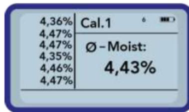
Six measurements in the "Average" operating mode already gives the user a representative measurement result for all the measuring points over a broad range of material.
