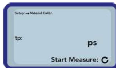
Four measurements are taken in order to increase the accuracy. An average of these measurement values is then calculated. The measuring time is approximately 20 seconds. When the measurement is finished, the measured pulse transit time is displayed briefly.
