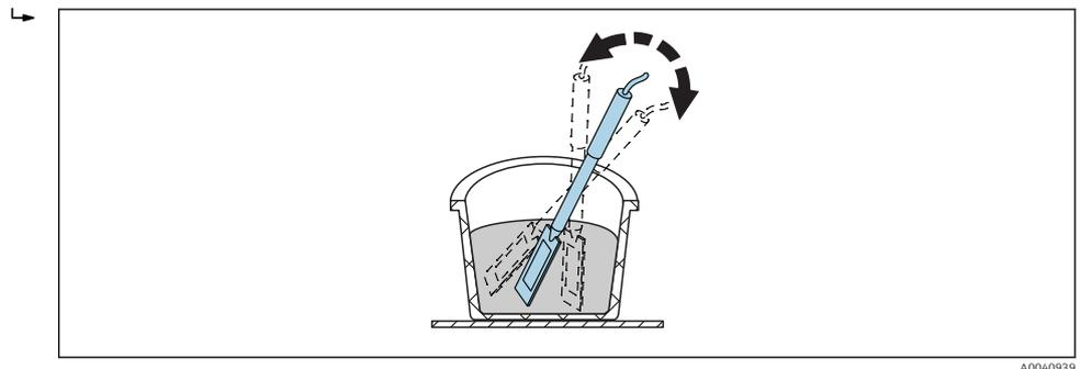
This ensures that a representative concrete mix is present around the surface of the probe.
