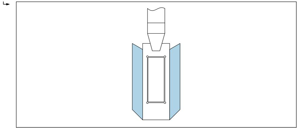
The plug-in blade ensures that the larger gravel pieces do not "drift away" from the probe head towards the side during the measurement, which can cause inaccuracies.
