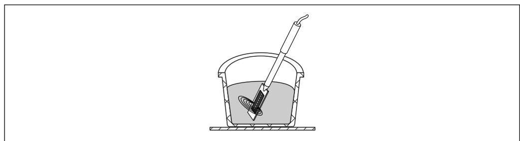
17 Measuring field propagation of the SWZ probe
