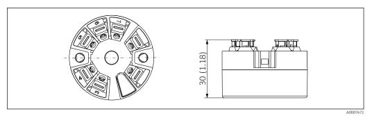
Version with push-in terminals. Dimensions are identical to the version with screw terminals, apart from housing height.
