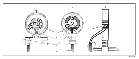
$\blacksquare 11$  Connecting the signal cables and power supply
