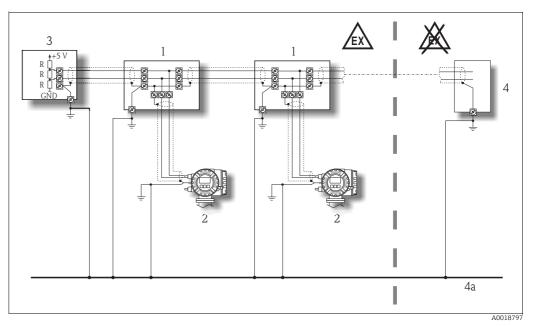
*Fig. 4: Example for connecting potential equalization lines*
