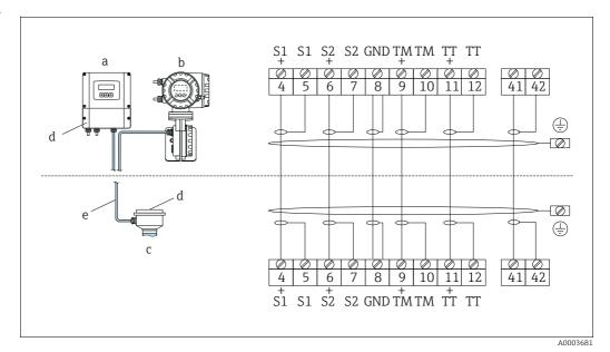
*Fig. 5: Connection of remote version connecting cable*
