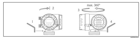
Fig. 1: Turning the transmitter housing
