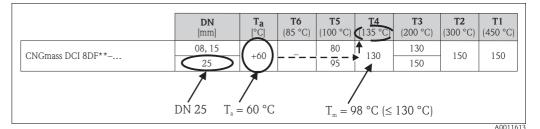
Fig. 2: Procedure for calculating the max. surface temperature
