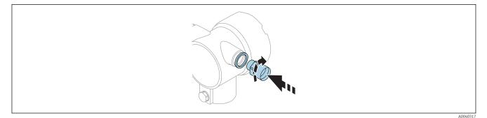
I Tighten the adapter/cable gland with the appropriate torque, see the table above.
