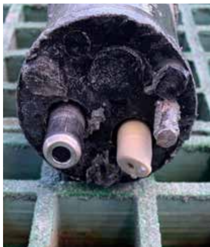
CPA111 with COS81D and CPS47D in cyanide leaching measuring point. Plastic protection stands are completely worn out but sensors are not.
