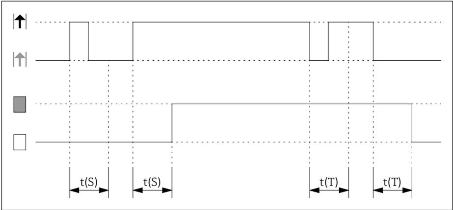
26 Adjustment of switching delays
