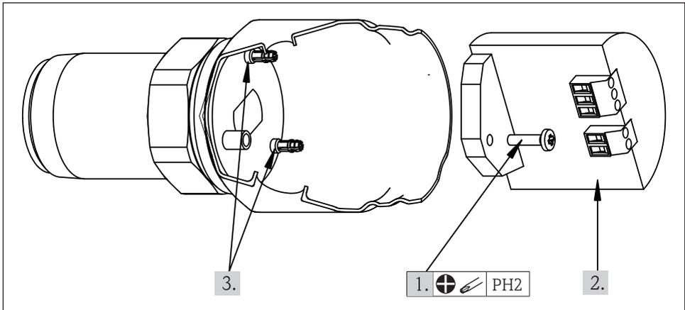
28 Replacing the electronics
