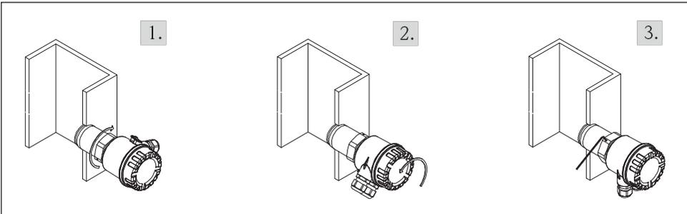
5 Installation with self-sealing connection thread
