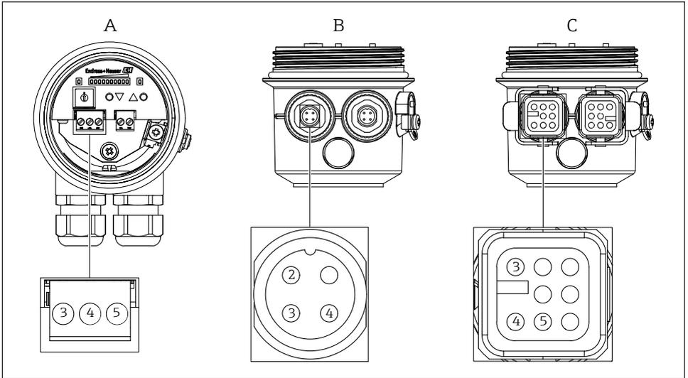
11 Signal output connection (connector 2)
