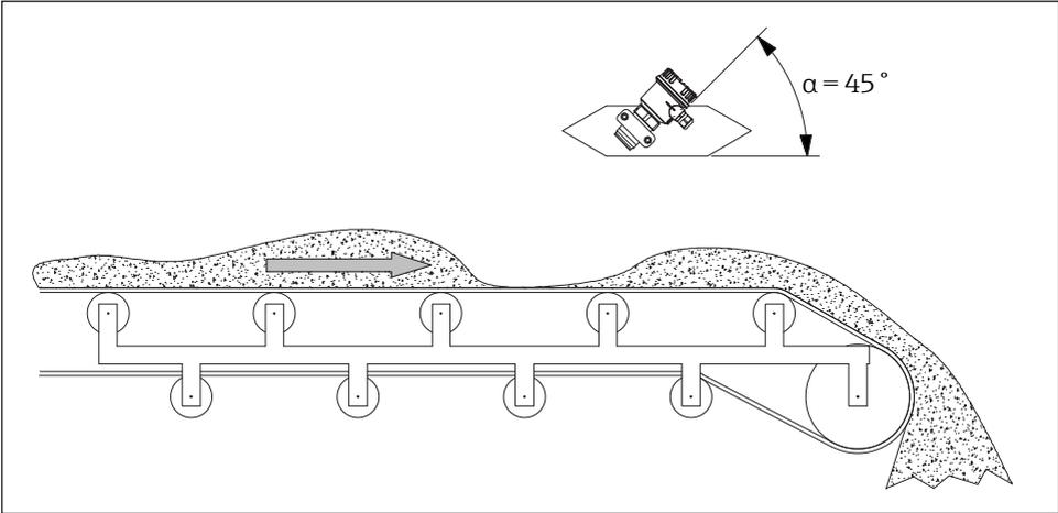
4 Installation position for material detection on conveyor belt
