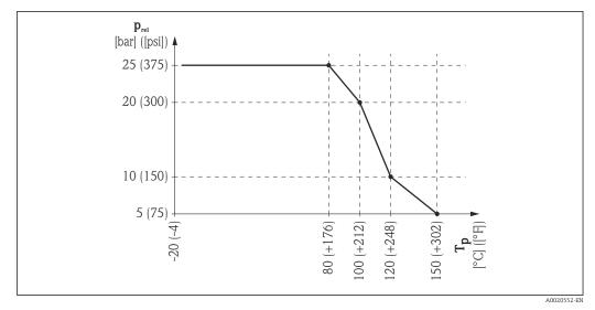
$\blacksquare$  25 FMR54 with planar antenna: Permitted range for process temperature and process pressure
