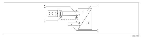
■ 13 Block diagram PROFIBUS PA / FOUNDATION Fieldbus
