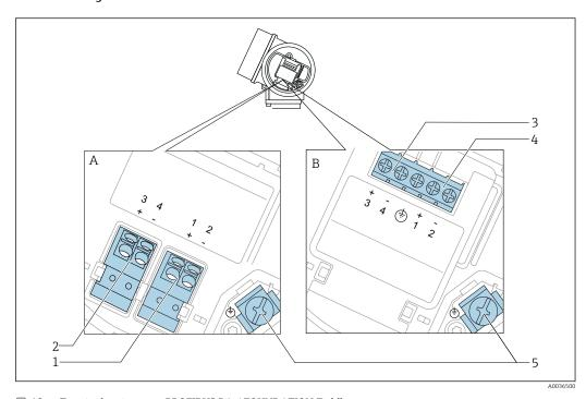
$\blacksquare$  12 Terminal assignment PROFIBUS PA / FOUNDATION Fieldbus
