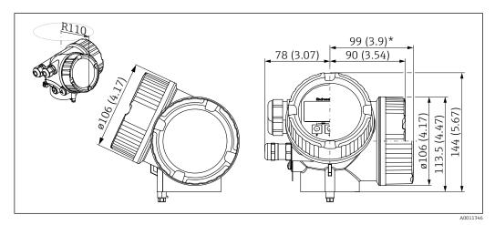
■ 27 GT19 housing (plastic PBT). Unit of measurement mm (in)
