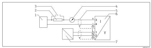
$\blacksquare$  11 Block diagram 4-wire: 4-20 mA HART (90 to 253  $V_{AC}$ )
