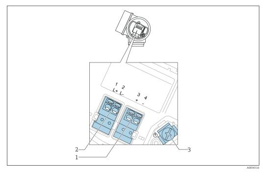
₽8 Terminal assignment 4-wire: 4-20 mA HART (10.4 to 48  $V_{DC}$ )
