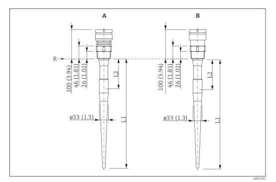
$\blacksquare$  30 Dimensions of device with thread. Unit of measurement mm (in)
