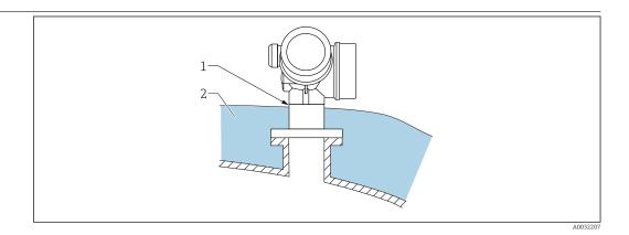
If process temperatures are high, the device should be included in the usual container insulation system (2) to prevent the electronics from heating as a result of thermal radiation or convection. The insulation should not be higher than the neck of the device (1).
