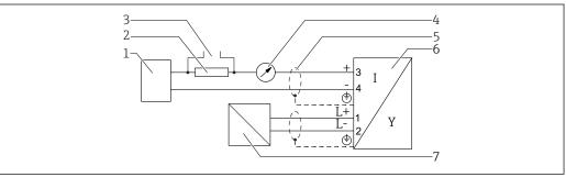
₹ 9 Block diagram 4-wire: 4-20 mA HART (10.4 to 48  $V_{DC}$ )
