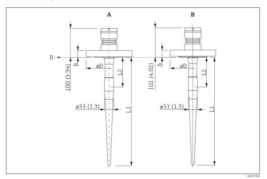
$\blacksquare$  29 Dimensions of device with flange. Unit of measurement mm (in)
