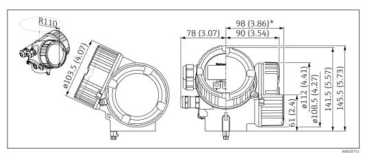
■ 28 Housing GT20 (aluminum coated). Unit of measurement mm (in)
