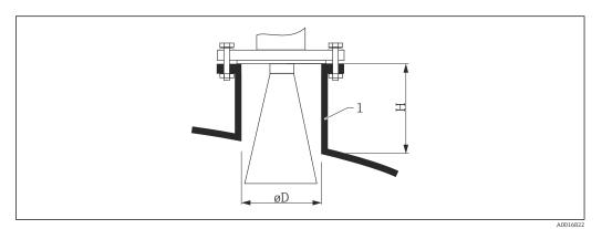
$\blacksquare$  20 Nozzle height and diameter for horn antenna
