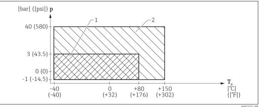
FMR53: Permitted range for process temperature and process pressure
