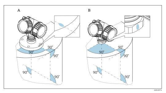
Depending on the device version the marking may be a circle or two parallel lines.
