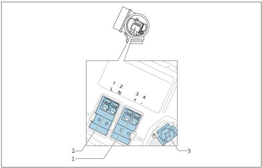
Terminal assignment 4-wire: 4-20 mA HART (90 to 253  $V_{AC}$ )
