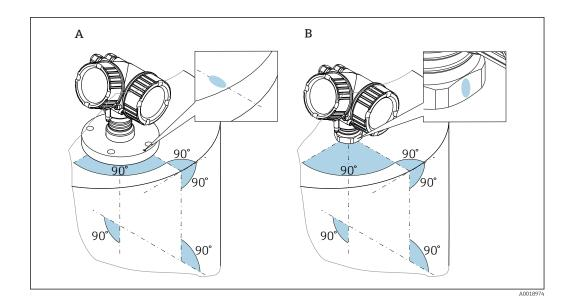
Pepending on the device version the marking may be a circle or two parallel lines.
