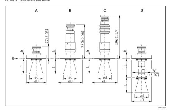
$\blacksquare$  31 Dimensions of FMR54 with horn antenna. Unit of measurement mm (in)
