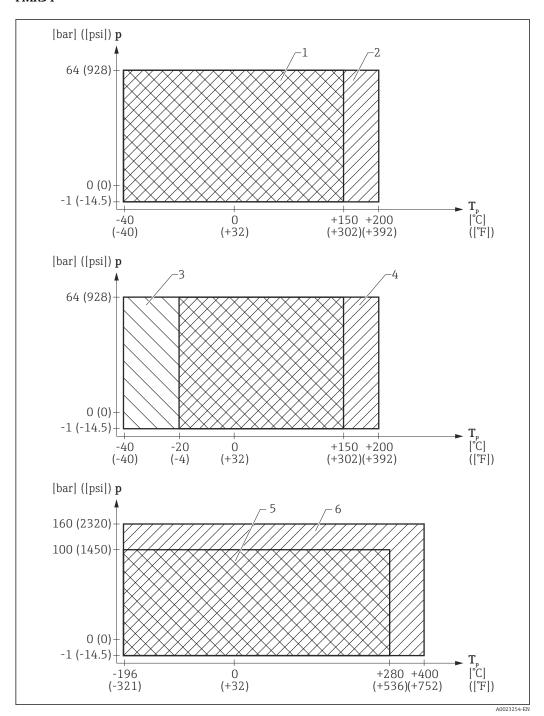
$\blacksquare$  24 FMR54 with horn antenna: Permitted range for process temperature and process pressure
