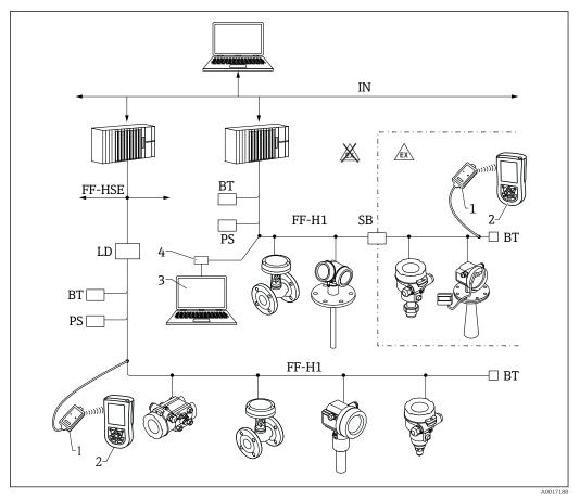
FOUNDATION Fieldbus system architecture with associated components
