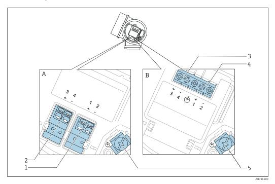
■ 6 Terminal assignment 2-wire: 4-20 mA HART, 4-20 mA
