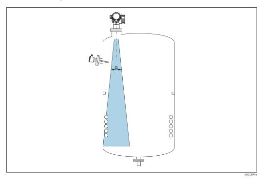
Avoid the location of internal fittings (limit switches, temperature sensors, struts, vacuum rings, heating coils, baffles etc.) inside the signal beam. Take the beam angle into account.
