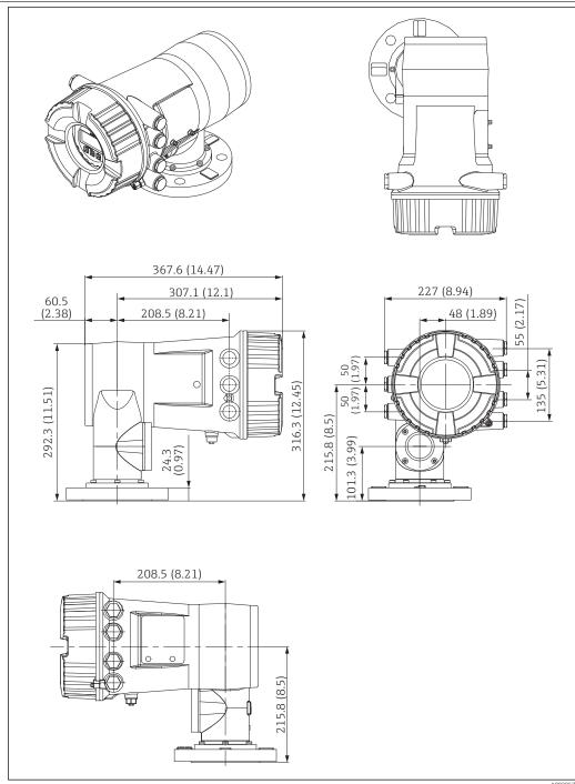
The thickness of the flange (24.3 mm (0.96 in)) shows the specification of the NPS 3" Cl. 150 RF, Alu flange ASME B16.5.
