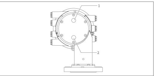
$\blacksquare$  28 Holes for cleaning nozzle and gas purging nozzle
