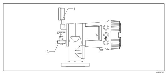
27 Mounting position of relief valve and pressure gauge
