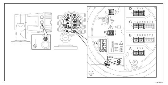
■ 11 Terminal compartment (typical example) and ground terminals
