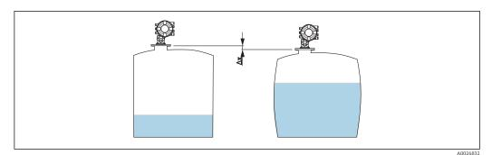
$\blacksquare$  23 Movement  $\Delta x$  of the tank reference height due to the bulging of the tank shell caused by hydrostatic pressure
