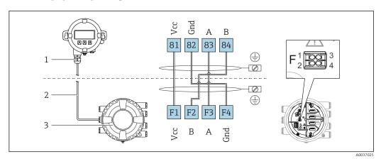
2 13 Connection of the remote display and operating module DKX001 to the Tank Gauging device (NMR8x, NMS8x or NRF8x)
