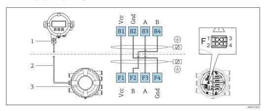
13 Connection of the remote display and operating module DKX001 to the Tank Gauging device (NMR8x, NMS8x or NRF8x)
