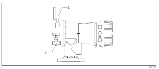
**2**7 **2**7 Mounting position of relief valve and pressure gauge
