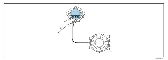
■ 20 Operation via remote display and operating module DKX001
