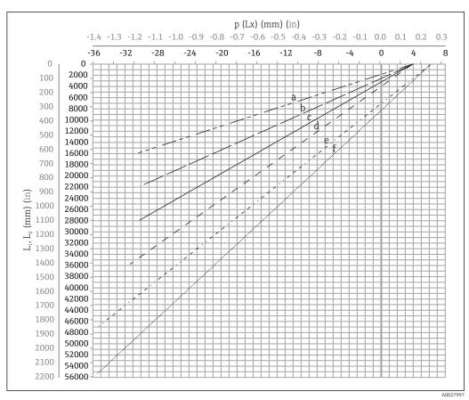
■ 16 Lateral shift of displacer according to measurement range
