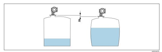
■ 23 Movement  $\Delta x$  of the tank reference height due to the bulging of the tank shell caused by hydrostatic pressure
