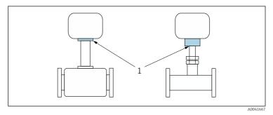
Position of reference point for temperature measurement
